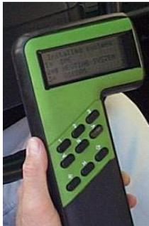
Later Bosch marketed the more advanced KTS300 (Porsche 9288) which became famous under the name of the Bosch "Hammer" because of its shape. This is a more versatile tool than the 9268 and was able to provide test signals, information, check sensor signals, and read fault codes from several models and controllers.
